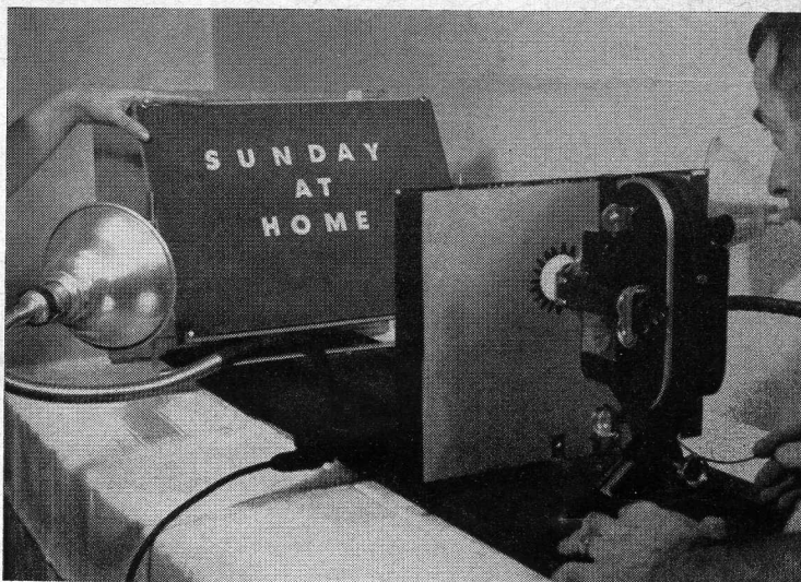
ASSISTANT is required to film a flopover title. Camera operator gives a signal at the desired time for flipping the board. Note cutout in front of lens to eliminate reflections from the camera.
