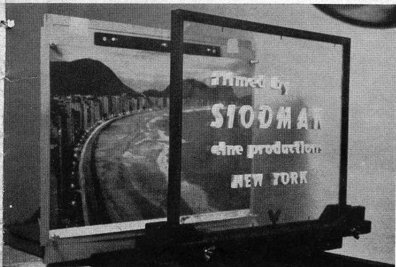
CALENDAR photo is used as a colorful background for the title. The letters are pasted right onto the glass, and the frame is held by special holder. Learn the way to avoid shadows from letters.
